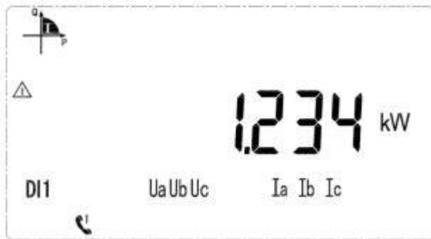
Current total power is 1.234kW
