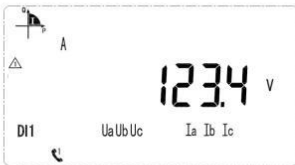
Voltage on A phase is 123.4V
