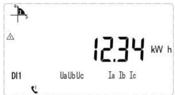
Current reversing active energy 12.34kWh
